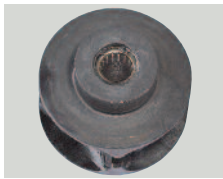
Load chain sheave with needle bearing
